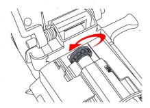
With hop up, BB pellets are able to extend its trajectory with revolution. Adjust with  $2\mbox{mm}$  wrench.
